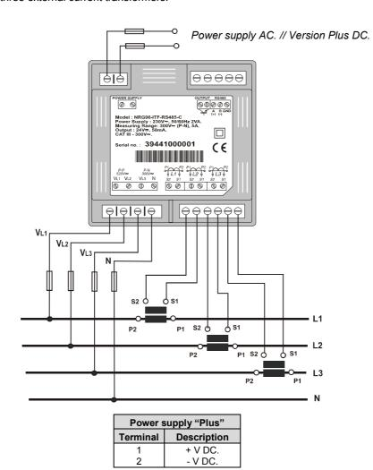
B. Three phase system measurement with 3 wire connection (Low Voltage) and three external current transformers.
