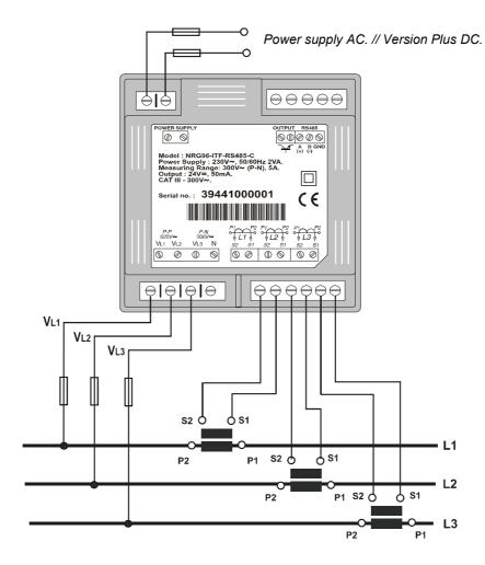
C. Three phase system measurement with 3 wire connection using 2 transformers and three external current transformers.
