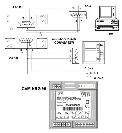
For communication with the master unit, the RS-232 to RS-485 System Protocol Intelligent Converter has to be used (M54020 Intelligent Converter). This converter does not require the 7 Pin connection in the RS232 part.
