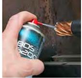
Step 1: Prior to drilling, spray high-performance lubrication spray directly into the drill.
