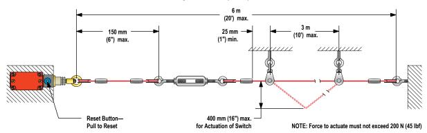
All hardware is supplied by the user. The switch mounting holes are on a standard limit switch mounting pattern of  $30 \times 60$  millimeters, and accept M5 (#10) hardware. Wire rope and associated hardware may be ordered separately; see Accessories on page 6.
