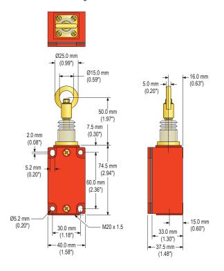
Figure 7. Model RP-LM40D-6L
