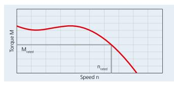
Constant smooth-start characteristics with no excessive starting and breakdown torque
