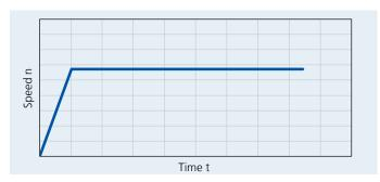
ZBE/ZNE motors are used for continuous duty applications
