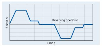
ZBF and KBF motors tend to be used for applications involving reversing duty with creep-positioning speeds.
