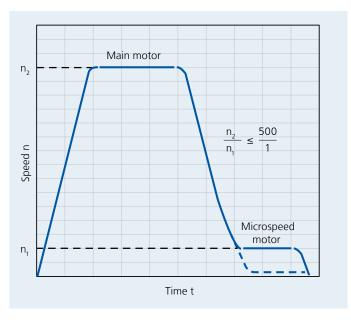
By selecting the right combination of motor and gearbox, the speed ratio can be set within a broad range
