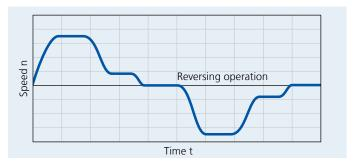
ZBA/ZNA motors tend to be used for applications involving reversing duty and creep positioning speeds
