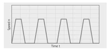
KBA motors are suitable for extremely high start-stop frequencies
