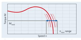
When using an inverter, it is possible to adjust the characteristic curve, which is optimized for travel applications
