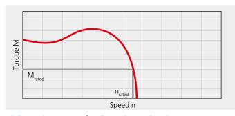
High starting torque for dynamic acceleration
